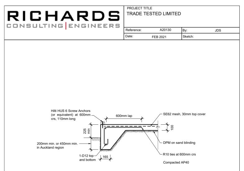
CONCRETE PERIMETER FOOTING SCALE 1:20
